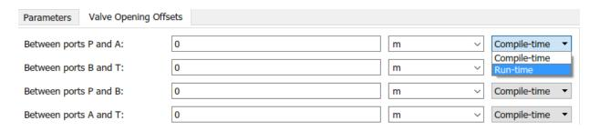
Compile-time parameters update in value only when you recompile the model. Use them when performing tasks that rely on inlined parameters such as model optimization. Run-time parameters update in value without the need for extra compilations. Use them when tuning parameter values in Fast Restart mode or when simulating models that rely at least in part on generated C code.
